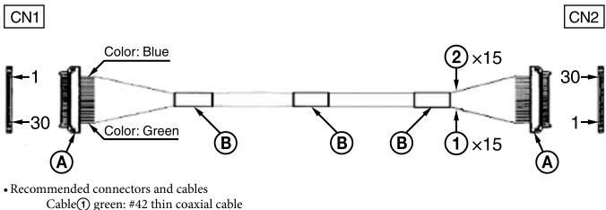
Cable(1) green: #42 thin coaxial cable Cable(2) blue: #42 thin coaxial cable Connector(A): USL20-30S (KEL) Binding tape(B)
